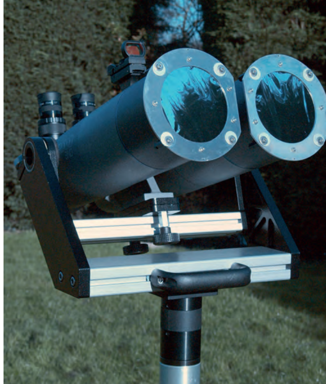
100mm 'four-posted' Euro EMC solar filters slide easily on to the exterior of the binoculars' dew tubes.
