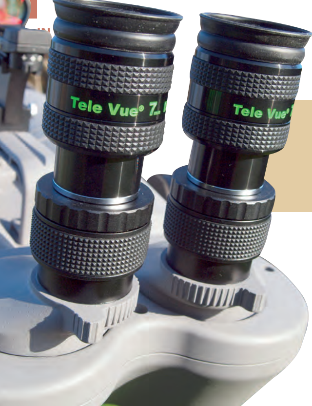
Eyepiece turrets, showing (from bottom up) the thumb-driven inter-ocular adjustment, knurled focusing rings and ridged eyepiece clamps.
